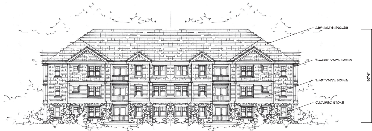
TYPICAL REAR ELEVATION 24 UNIT BLDG
