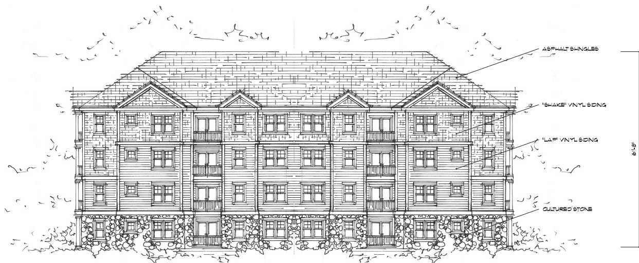
TYPICAL REAR ELEVATION 28 UNIT BLDG
