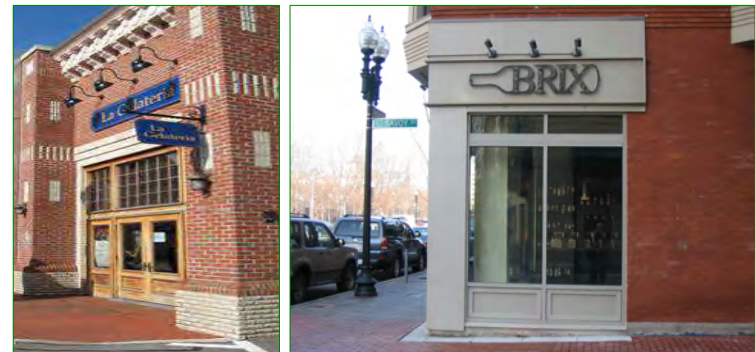
Primary signage is included in an externally-illuminated sign band, while a Blade Sign improves visibility to pedestrians.
