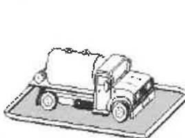
Several types of portable, temporary, synthetic drive-over mixing/loading pads are available commercially. Generally the pads are vinyl or nylon reinforced elastomer pads or steel pads and vary in size from 4 X 8 feet to 34 X 74 feet. Most have a flexible wall designed to be self-supporting. The material can be decontaminated. The pads are lightweight, easily deployed, durable and reusable.
